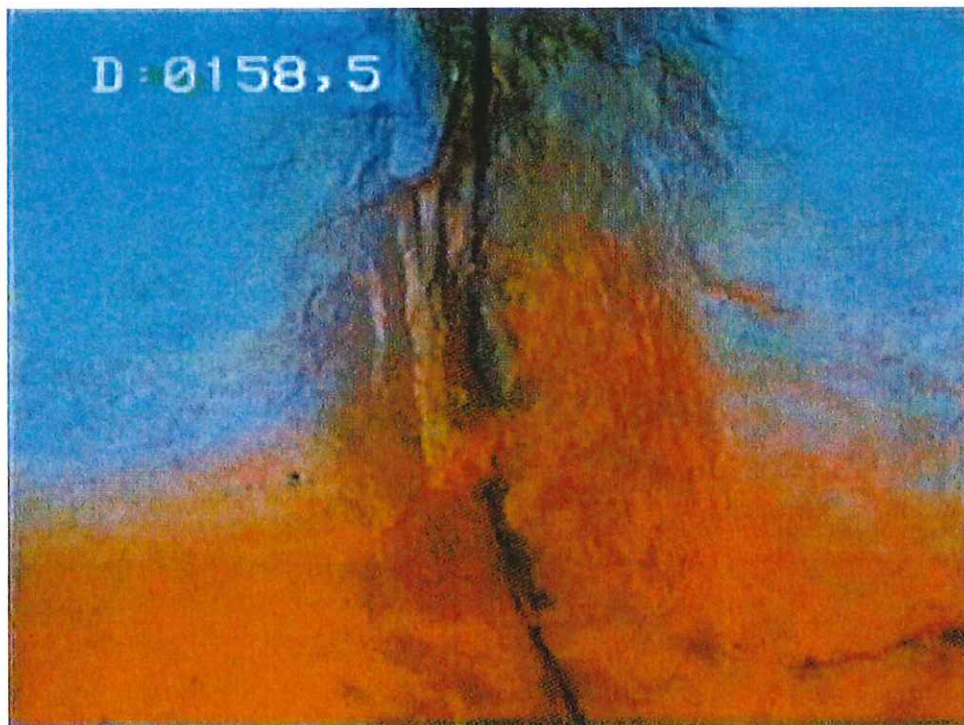
42- Trou nu – formation carbonatée massive, fracturation verticale
